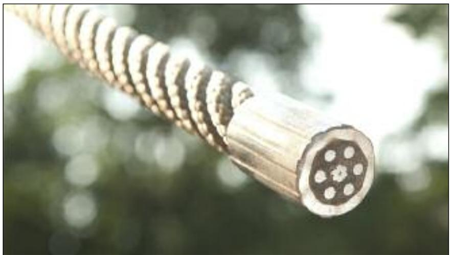
*This galvanized steel cable wrapped in a polyester yarn is typical 'rope' used for play equipment.*
